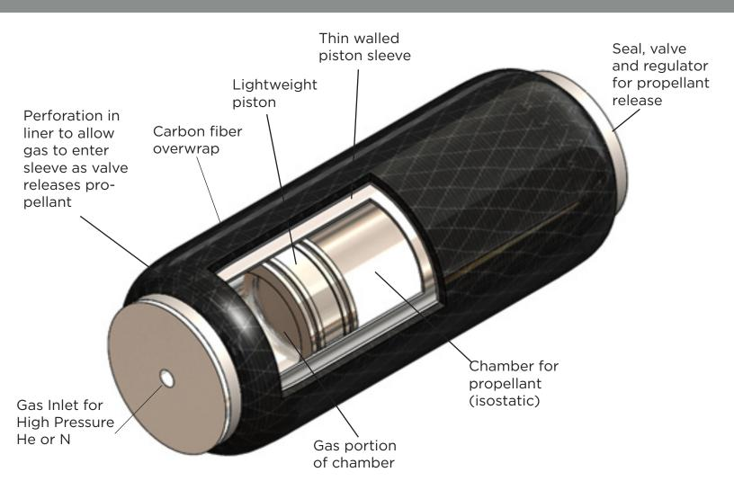
We have demonstrated a lightweight piston propellant system. The piston sleeve could be made of any material removing concerns about material compatibility, and since the sleeve is merely a barrier, could be made with very thin walls. The pressurant is housed in a high-pressure external chamber isolated from any propellant, but structural to the propellant chamber.
